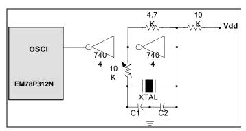
Fig. 5-32 Crystal/Resonator-Parallel Mode Circuit
